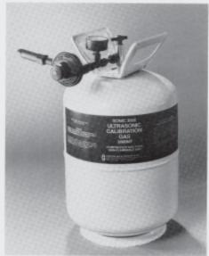
A standard method of calibrating the ultrasonic detector has been developed by the American Socity of Testing and Materials. By using the standard, leakage rates can be estimated, detectors can be uniformly regulated for particular functions, and repeatable results can be assured. Calibration can help you avoid mistakes and perform tests that previously required more expensive instruments.
