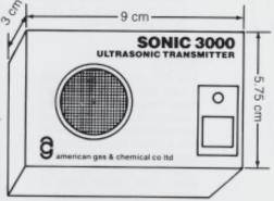
The generator transmits a distinctive ultrasonic signal in the 45 kilohertz region. The generator saturates an area with ultrasound which penetrates small holes and cracks. The air probe uses the escaping sound beams to home in on leaks. The generator is small enough to fit in small openings and powerful enough to make locating potential leaks easy. A light emitting diode flashes when the unit is in operation.
